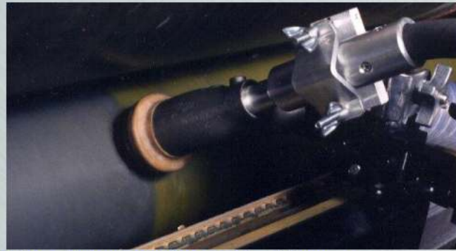
Anilox roll cleaning on flexographic printing press
