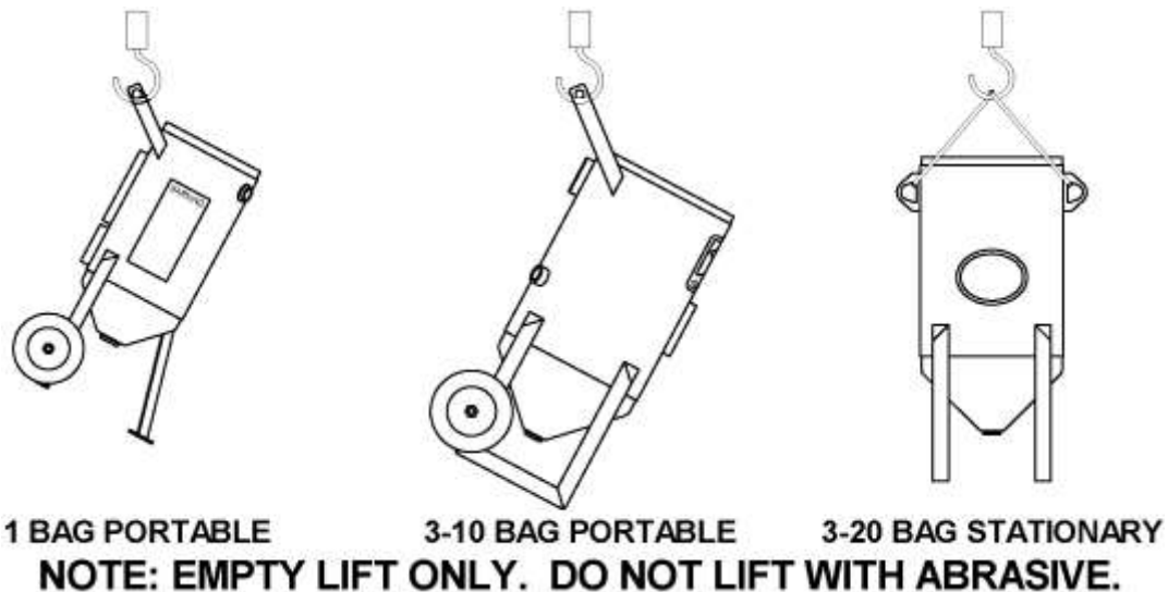
Figure 2.6(a) – Abrasive Blaster Lifting Diagram
