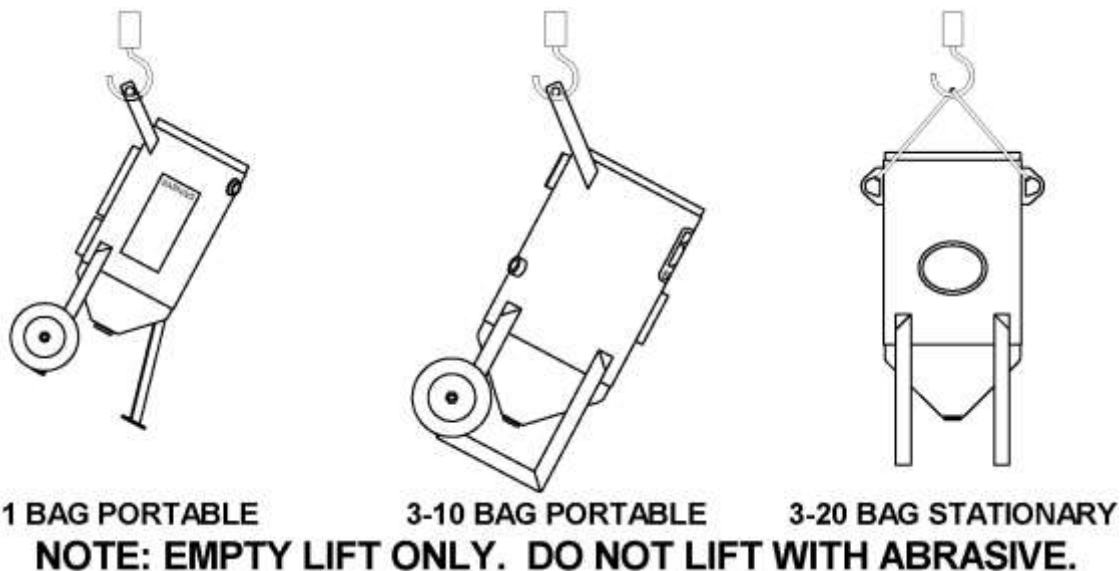
Figure 2.6(a) – Abrasive Blaster Lifting Diagram
